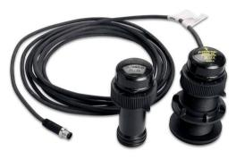
Includes blanking plug to allow active element to be removed for cleaning or maintenance. Skin fitting features a "self seal" flapper valve to minimise water ingress when transducer removed and blanking plug inserted.
