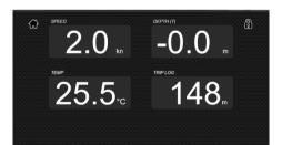
Simple digital displays of key instrument data – easily configurable for any value on the network If there's a chart plotter on multi function display on the NMEA 2000 network with active nav information such as a GOTO or route, iSeaSense will display current navigation data such as XTE, bearing and distance to waypoint.
